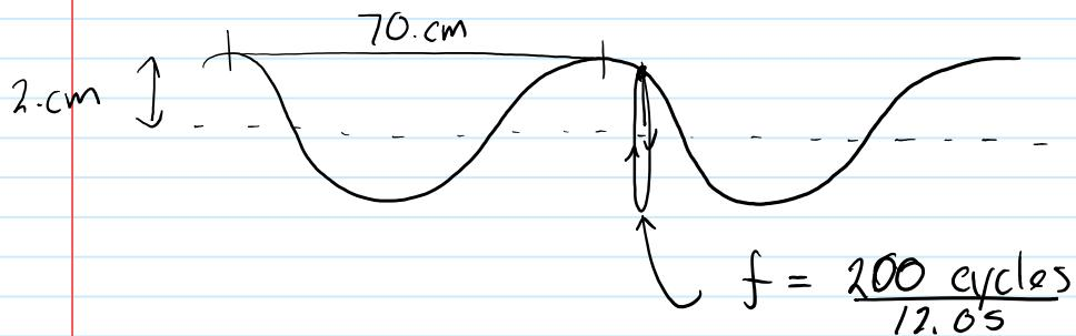
$$\text{a) } V = ? \quad V = \frac{\lambda}{T} \quad T = \frac{12.05}{200 \text{ cycles}} \quad \lambda = 70.0 \text{ cm}$$
